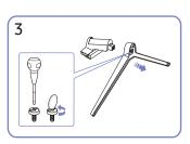
Remove the stand neck from the stand base by pulling it in the direction of the arrow as shown in the figure.
